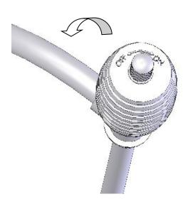
Exercise various pressures on the siphon bulb > Finish filling the fireplace tank, turn the knob off, turn it anticlockwise. This way you empty the siphon pump.
