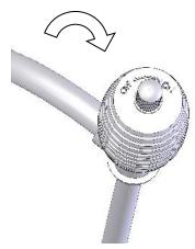
Turn clockwise (ON position) the knob at the > Dip the rigid pipe inside the bioethanol tank and top.
