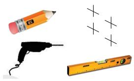
Mark the 4 holes positions with the aid support bracked; and proceed with drilling and inserting appropriate dowels to the type of wall;
