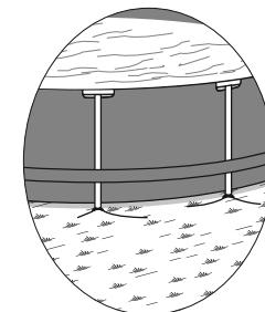
Do not assemble with pool legs on soft lawn. If you must assemble the pool on a soft surface, timber boards (not included) must be placed under the feet of the vertical support rods for even weight distribution.
