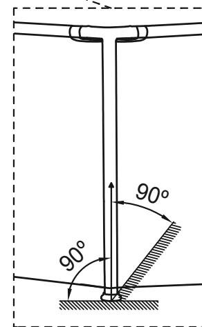
After the installation of the pool's steel frame is completed, ensure that the verticals are perpendicular to the ground. If they aren't, the verticals could be bent or deformed.
