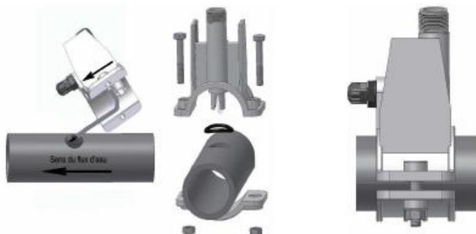
Installation of 4 x 6 tube (ref. 2) on d e f g elements
