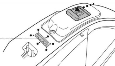
3. Immerse the robot into the water and operation will automatically begin as water level covers the sensors at the top of the swivel head. Let the robot sink to the pool floor and observe the cleaner's first forward and reversed movements across the pool bottom. If the robot runs along the pool wall instead of perpendicular to it, reposition it to make sure that its front/back faces the pool wall.
