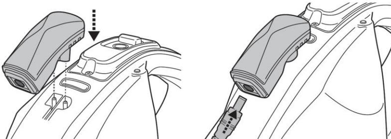
3. Connect the external adaptor to the power source. Once the robot begins charging, the indicator light on the external adaptor will turn red. The indicator light on the external adaptor will turn green when the robot is charged. Charge it for 5-6 hours for best performance.
