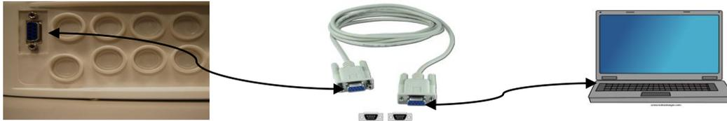
You can use an RS232→USB adaptor if the PC has no serial ports. In order for the devices to communicate, it is necessary to use a null modem serial cable, or a straight serial cable with a null modem adaptor.
