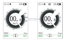
(6) "SOC View" --- set display mode for battery level
