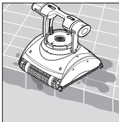
Place the Pool Cleaner on the edge of the pool and let the water drain out.
