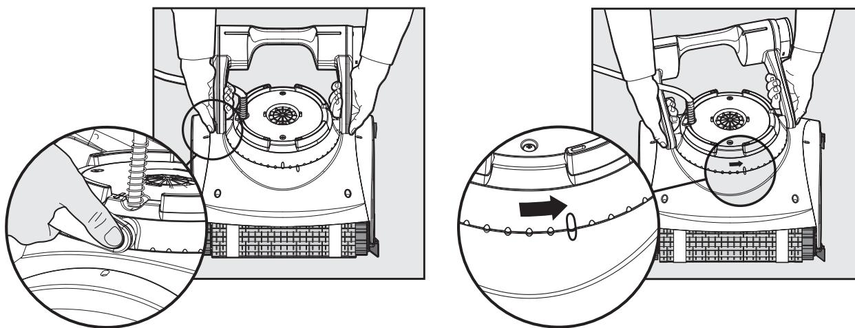
While pushing the button on each float, pull it all the way out.
