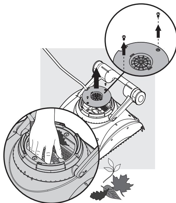
If you notice debris trapped in the impeller, open the impeller and remove the debris.
