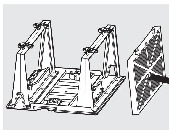
Open the clips and remove the filters.
