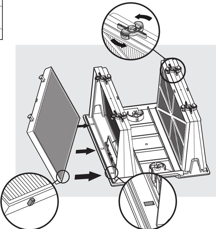
Insert the filters with the plastic backing facing out.
