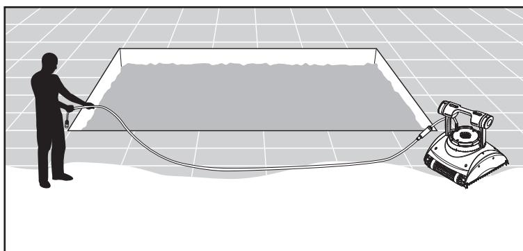
Unwind the cable and stretch it out completely so that it has no kinks.
