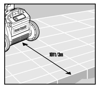
Position the power supply so that it is in the approximate middle of the long side of the pool at a distance of 3m (10ft) from the edge of the pool.
