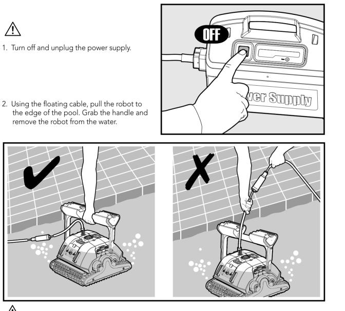
DO NOT PULL THE ROBOT OUT OF THE POOL USING THE CABLE.
