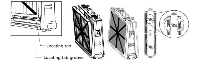
Reinstall the base frames with filters according to the diagram.
