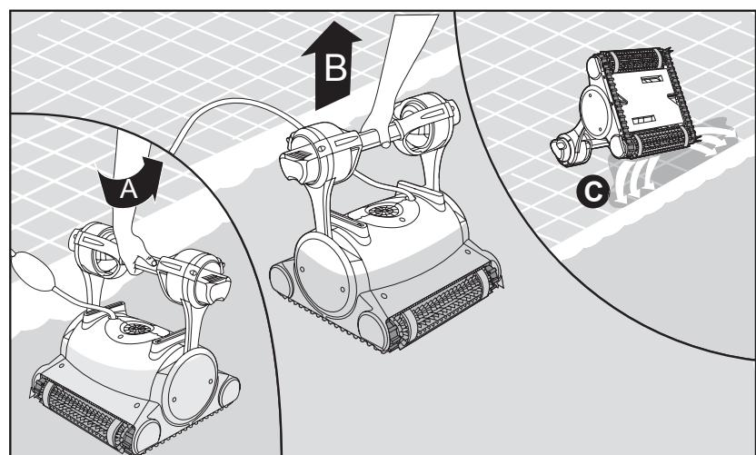
Using the floating cable, bring the Pool Cleaner to the pool's edge.
