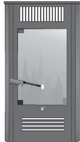
APPROACH THE LIGHTER TIP NEAR THE BIOETHANOL WITHOUT TOUCHING THE COMBUSTIBLE
