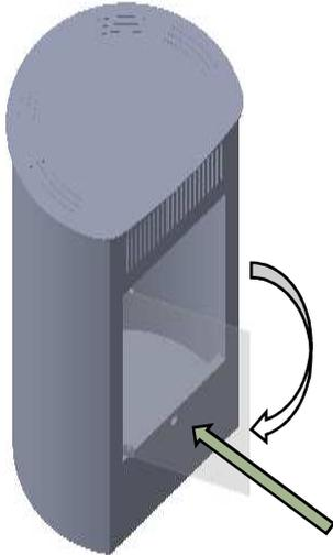
Close the tank by operating on the regulation rod (c), gently close the glass door
