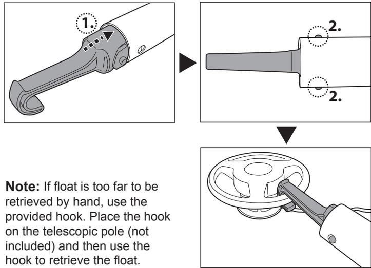
**Note:** If float is too far to be retrieved by hand, use the provided hook. Place the hook on the telescopic pole (not included) and then use the hook to retrieve the float.
