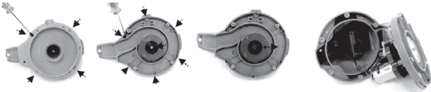
3. Remove the battery pack to expose the PCBA. To detach the battery connection wire, press the clip on the connector and then pull it out. **NOTE:** Wrap the connector immediately with insulating tape in order to avoid short circuit caused by contact of both wire terminals.
