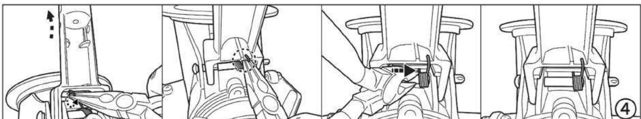
4. Use a pair of pliers to pull the hook from the bottom of the connector, then fix it onto the connector as shown. Move the entire spring to the right.
