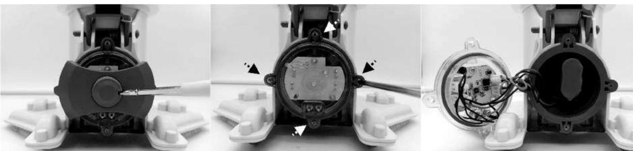
2. Remove the battery from the unit and locate the battery cable connector. Press on the clip of the connector to pull it out. NOTE: Wrap the connector immediately with insulating tape in order to avoid any short circuit caused by the contact of both wire terminals.
