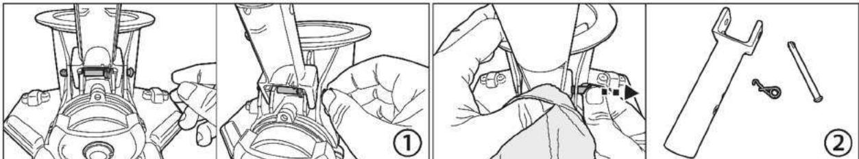
1. Grasp the top round end of the pin. Use a pair of pliers to help with removal if necessary.
