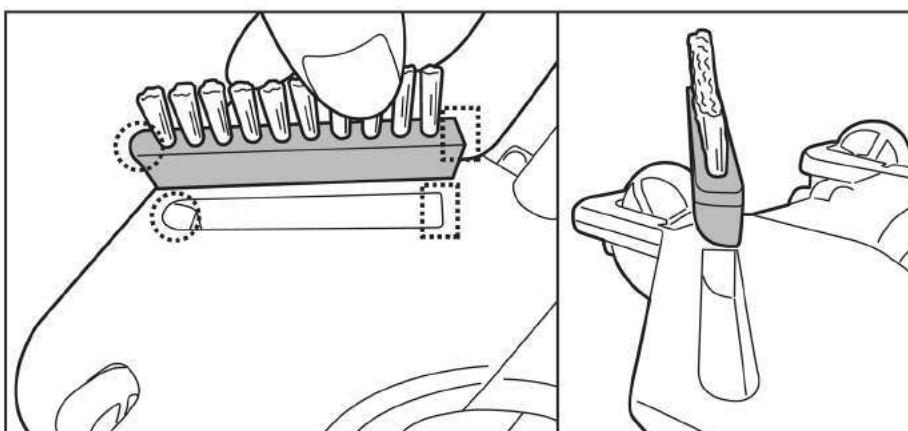
To detach the brush, insert the tip of a small screwdriver into the corner notch and pry up the brush.
