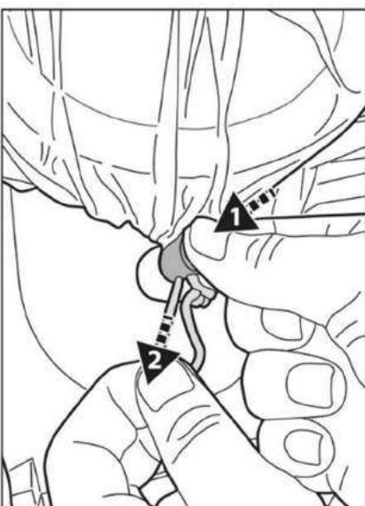
While holding the cord, press on the cord fastener and push it under the flange.
