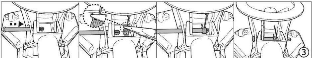
3. Insert the pin from one end and place the spring as shown with the help of a pair of pliers. Ensure the hook is on top and the other end is installed underneath the bench as shown. Align and insert the pin all the way through the spring hole and opposite hole.
