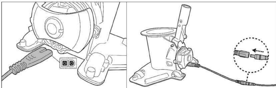
3. Connect the external adaptor to the power source. The indicator light on the external adaptor will turn red when the vacuum is charging and green when it is fully charged. Charge it for 5-6 hours for best performance.
