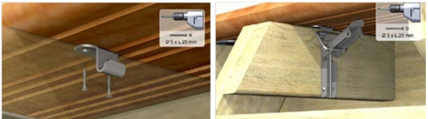
Figure 38 – Assembly of the hook/ lever lock system
