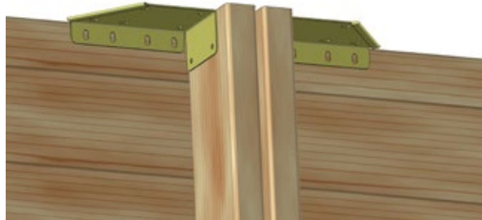
Figure 18 – Fastening metallic support brackets to the top of the supporting braces
