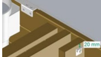
Figure 35 – Location of the lock striking plate
