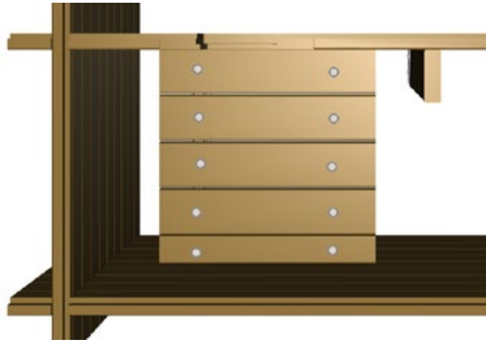
Figure 15 – Assembling the base of the plant housing portion of the box
