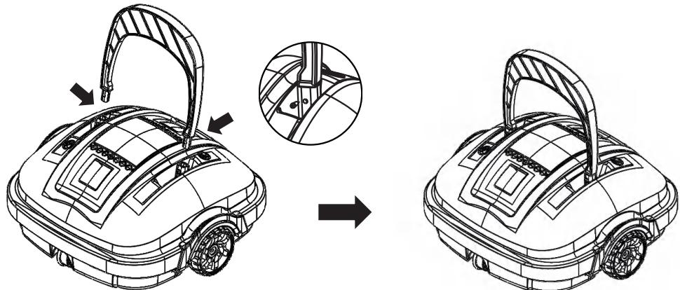
Note: The installation direction of 2 screws is opposite.
