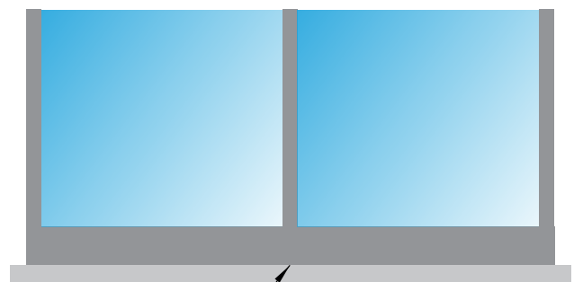
Fig. 2. Non-suitable surface for proper functioning - pool enclosure doesn't work
